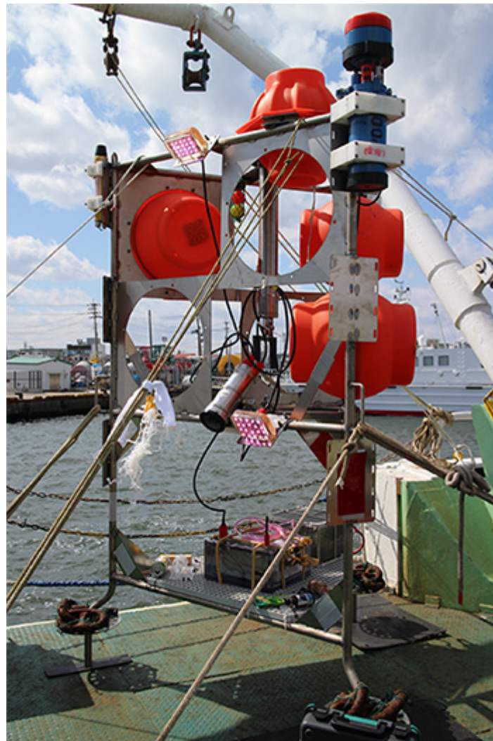
Figure 1: A deep-sea station used for the monitoring. The installed instruments are (1) ARGOS satellite transmitter, (2) RDCP 600, acoustic doppler current profiler, CTDDO-turbidity sensors with battery, (3) LED lights, (4) ROV homer, (5) glass spheres, (6) acoustic release transponder, (7) HDTV camera in a stainless pressure cylinder, and (8) oil-filled Lithium-ion battery for the camera and the lights.
