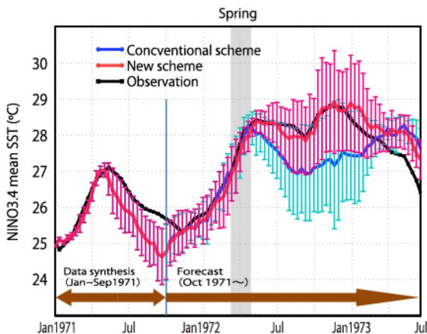
Figure 1: Predicted NINO 3.4 (5°N–5°S and 170°–120°W) SST (sea surface temperature) anomaly (red and blue curve) as compared with observed SST anomaly (black). The values are for hindcast experiments during 1971–1973 derived from the conventional case without seasonal control (blue) and the new case using a seasonal adjustment factor (red). Grey shaded regions denote the boreal spring periods.
