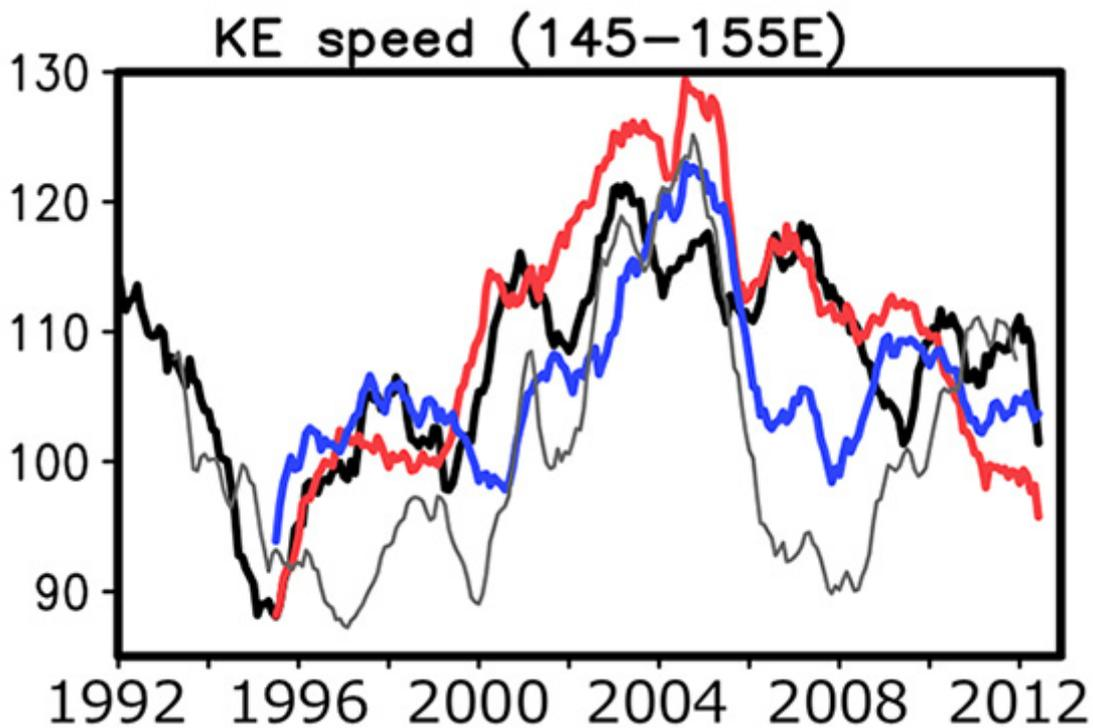
Figure 3: Time series of the Kuroshio Extension (KE) jet speed averaged over 145–155 °E, which was reproduced in three simulations shown in the figure 1 (black line, red line, blue line). The gray line shows satellite observations. To reduce impacts from ocean eddies and highlight interannual variability of ocean currents, 13-month running mean is applied to the time series of the KE jet speed.
