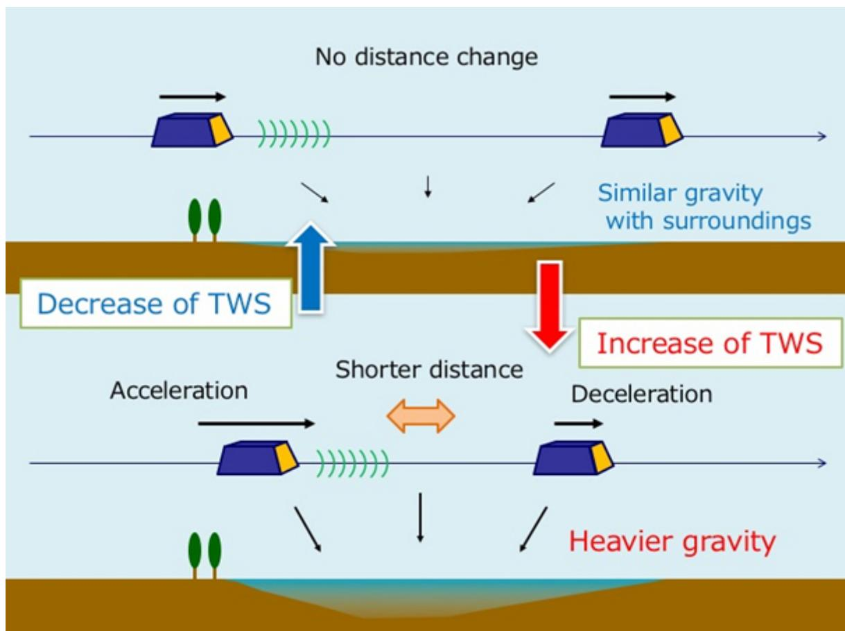
Figure 3. Measurement of terrestrial water storage by GRACE
