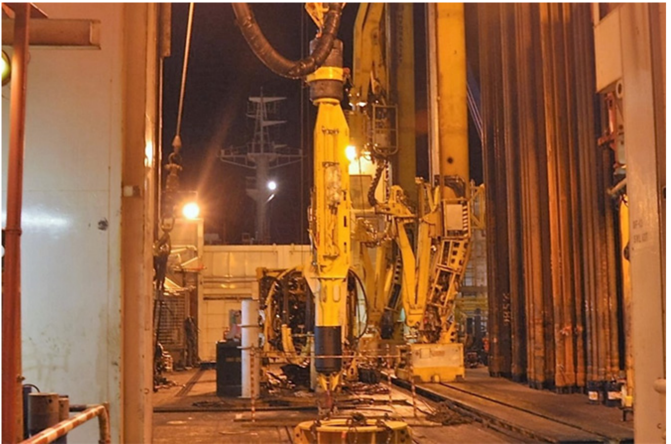
Figure 5. The borehole temperature observatory wellhead, which is connected to a drill pipe to install the observatory into the cased borehole where core samples were previously collected.
