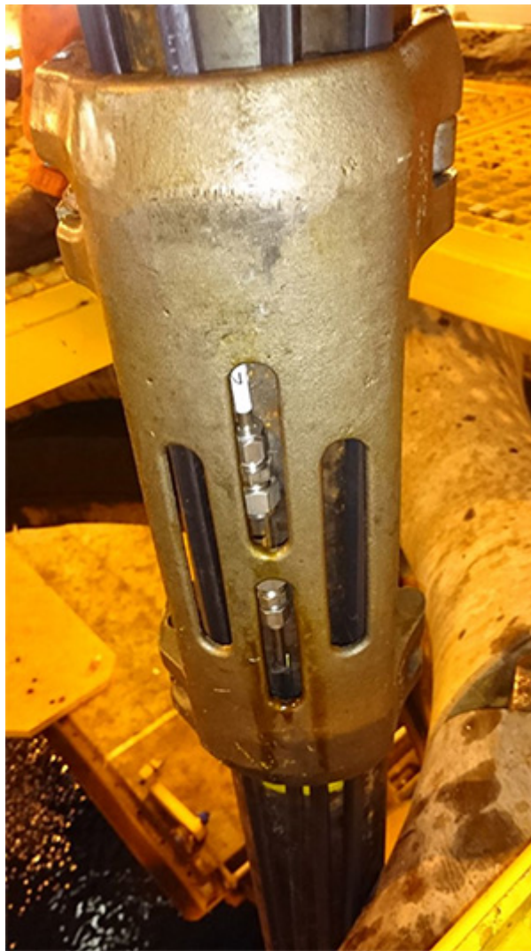
Figure 4. Temperature sensors used in this expedition; a total of 13 sensors were installed in the borehole (Hole C0023A).
