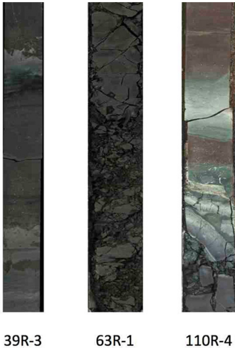
Figure 3. Core samples of sediments recovered from the deep subseafloor, representing lithological features in the Nankai accretionary complex off Muroto. From left: Core 39R-3, volcanic sandstones from 614 m below the seafloor; Core 63R-1, a décollement fault (a horizontal fault which is identified as the plate boundary in this case) including a brecciated zone from 758 m below the seafloor; Core 110R-4, a pelagic clay layer on top with altered basalts below, from 1125 m below the seafloor.
