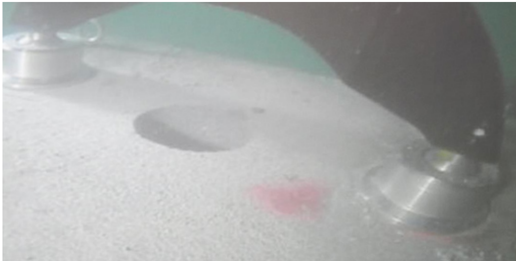
a. Removing a core sample from the test rock on the seabed
