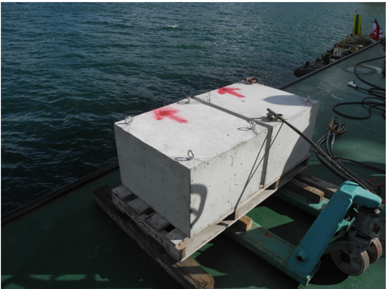
Figure 7. A test rock used in the drilling tests (made of mortar)
