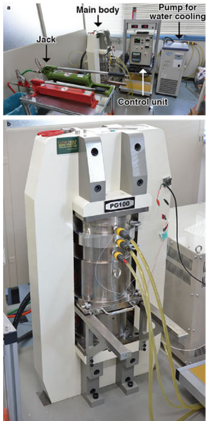
Figure 4. Boyd-England-type 1/2-in-diameter piston-cylinder apparatus used for the melting experiments at Kyoto University.
