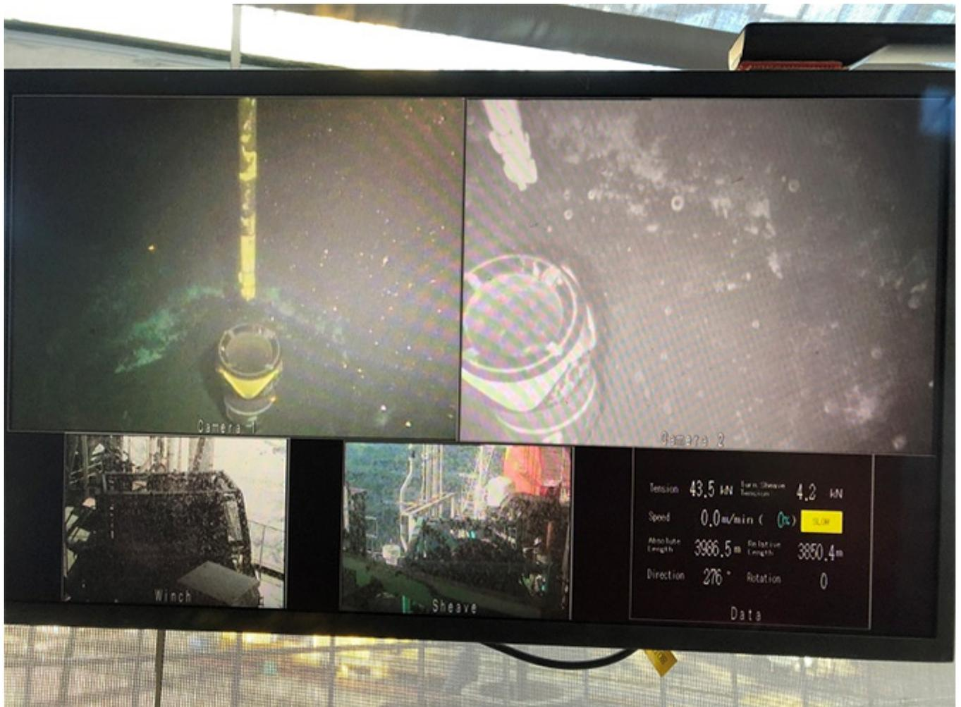
Photo 1: Re-entry process of drill pipes (taken by underwater camera)
