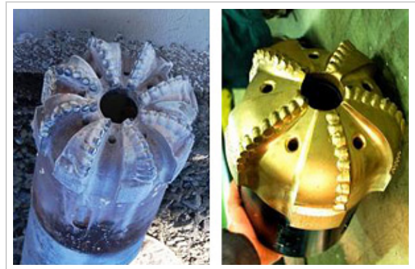
RCB core bit used in the NanTroSEIZE Stage1 (left) and newly designed bit (right). Sample recovery and quality are significantly improved.
