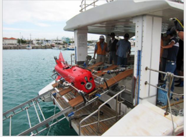
Testing of the newly-developed deployment and retrieval system for PICASSO-1. This is the first time PICASSO has been deployed from a ship without an A-frame, davit or crane. The aft hydraulic platform was slowly lowered while letting out the ropes to give PICASSO-1 a soft landing into the ocean. With this system it has become possible to deploy PICASSO from any ship around the world with an aft hydraulic platform. Surveys off the Great Barrier Reef in Australia are planned for next year.
