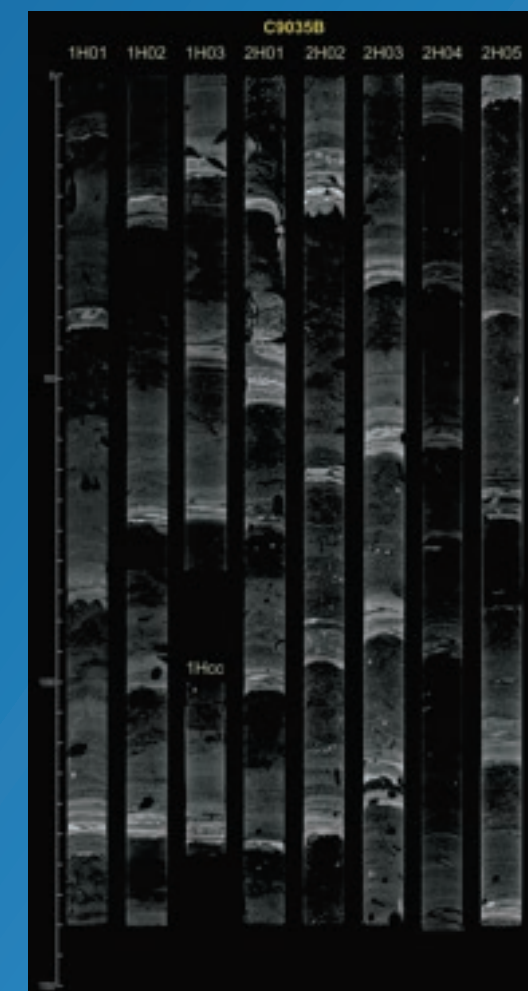
X-ray CT images of a core sample taken from the Nankai Trough.
