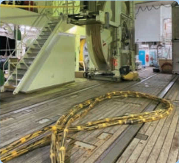
A hydrophone streamer cable. A number of hydrophones are placed every few meters. The cable length depends on the situation and can be more than 6km.
