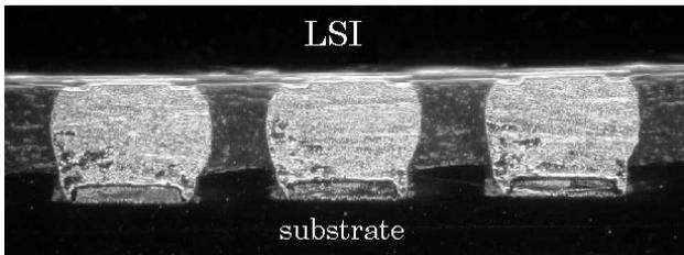
Photo 4 Cross section of solder joint between substrate and bare chip.
