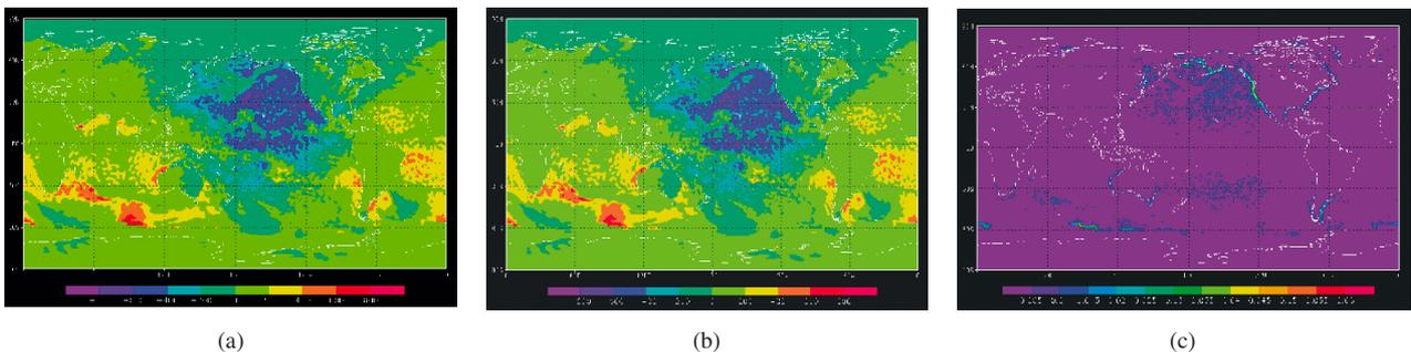
Fig. 2 Residual estimation between AFES component with T106 and OFES component with half of T106 resolution. (a): Three hours averaged heat flux distribution data from AFES component, which was used as input data before interpolation, (b): data obtained from OFES component after interpolation, and (c) shows residual between AFES (a) and OFES (b). Residual was converted on AFES grid system.
