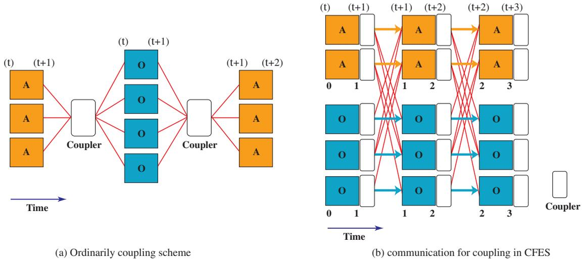
Fig. 1 Structure of coupling interface between atmospheric and ocean GCMs.
