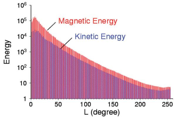
Fig. 1 Energy spectra obtained from a numerical simulation of magnetoconvection at  $E = 10^{-5}$  and  $Ra = 2 \times 10^8$ . Red and blue bars show magnetic and kinetic energies in the fluid shell as functions of degrees of spherical harmonics.
