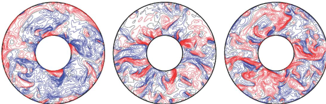
Fig. 2 A snapshot of magnetoconvection at  $E = 10^{-5}$  and  $Ra = 2 \times 10^8$ . From left to right, zonal velocity, radial velocity and axial magnetic field in the equatorial plane are mapped as viewed from the north, a red (blue) contour line showing a positive (negative) value.
