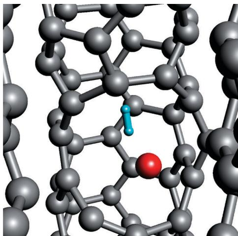
Fig. 4 Cleaning process for CNT. Optical excitation locally breaks C-O bonds and extract O atoms from carbon nanotubes. Red sphere and blue spheres show O atom and  $H_2$  molecules, respectively.
