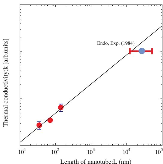
Fig. 1 Length dependence of thermal conductivity in CNT.
