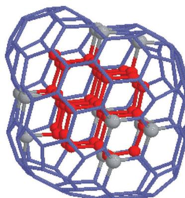
Fig. 3 Reconstruction of diamond nanoparticle into fullerene-like structure.
