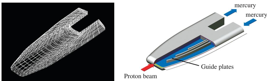
Fig. 1 Mercury target over view
