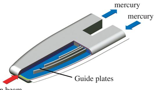
Fig. 1 Mercury target over view
