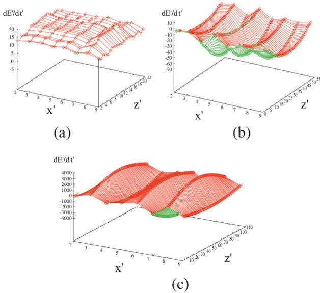
Fig. 2 Displacement current in IJJ by preliminary models simulation.  $t'=3.5$ ,  $x'$  axis: parallel to  $ab$ -plane,  $z'$  axis: parallel to  $c$  axis,  $\frac{dE'}{dt'}$ : displacement current to  $z'$  axis,  $\beta=0.03$ ,  $\alpha=0.1$ ,  $\gamma=0.1$ , the external constant current  $I'=1.04$  in this simulation. (a) 20 junction (b) 50 junctions (c) 100 junctions.
