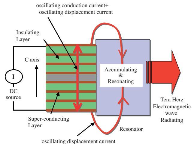
Fig. 1 Schematic diagram of antenna radiation model.
