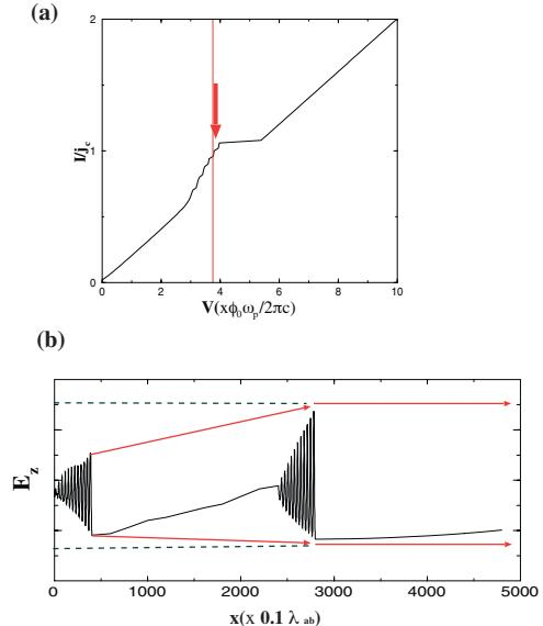
Fig. 3 (a)The I-V characteristics for the system of the junction array embedded inside a wave guide.(b) The snapshot of the spatial distribution of the electric field excited in the system.
