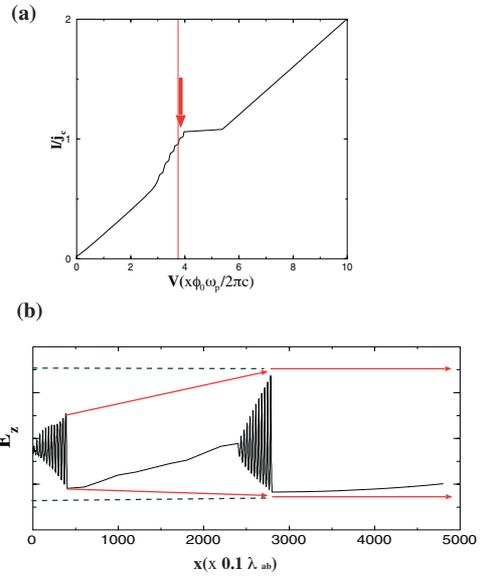
Fig. 3 (a) The I-V characteristics for the system of the junction array embedded inside a wave guide. (b) The snapshot of the spatial distribution of the electric field excited in the system.
