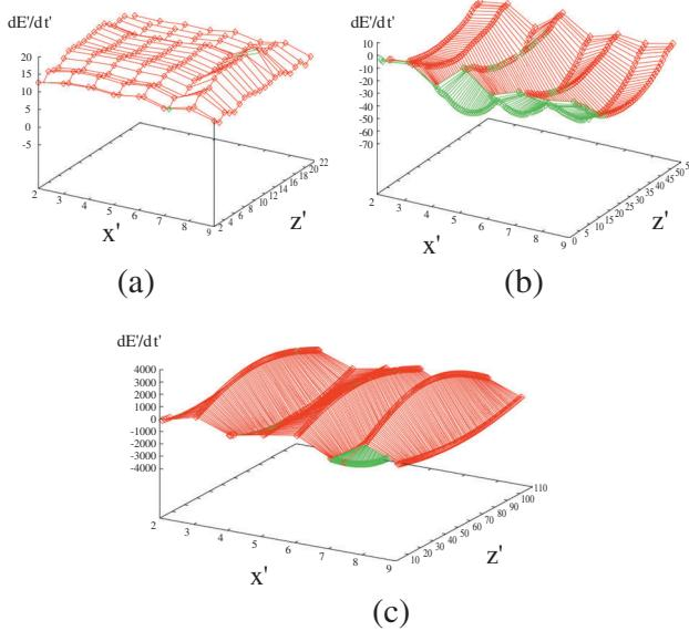
Fig. 2 Displacement current in IJJ by preliminary models simulation.
