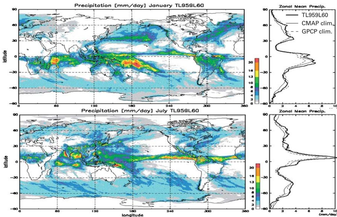
Fig. 1 The horizontal distribution of monthly-mean precipitation of January (top) and July (bottom) obtained from an integration at TL959L60 using climatological SST data as the boundary condition. The zonal mean precipitation of the model (thick solid line) and the climatological estimates of CMAP (thin solid line) / GPCP (thin dashed line) are plotted on the right panels. Units are mm/day.
