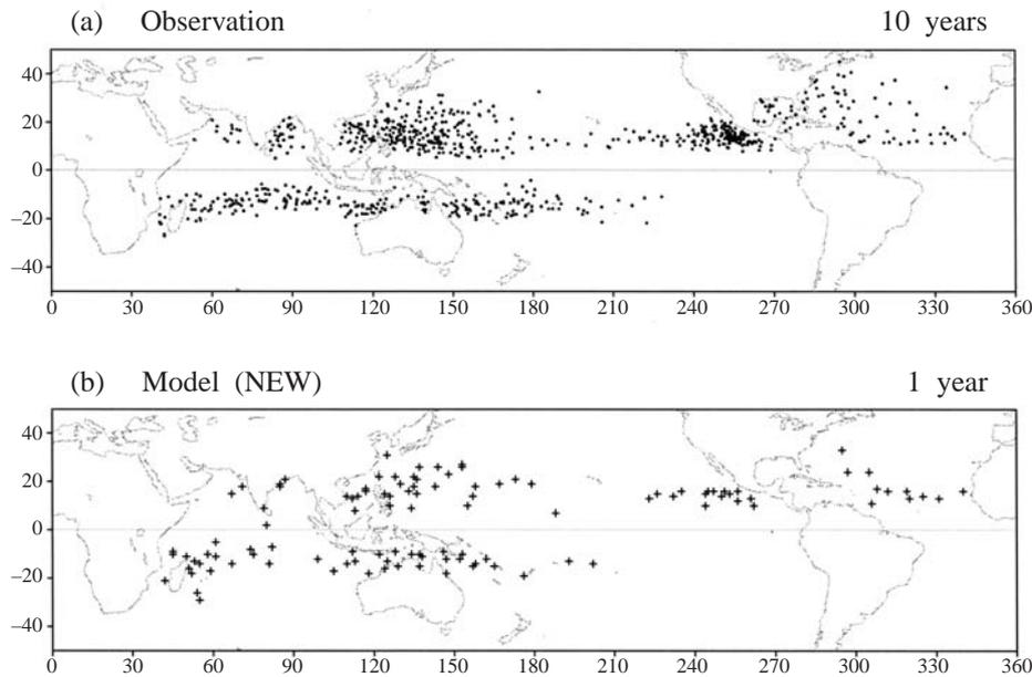
Fig. 2 (a) The location of origins of tropical cyclones by the observational data for 10 years (1979–1988). The points where cyclones grow up to have their wind speeds (sea surface) more than 17 m/s (34 kt) are plotted. (b) Those obtained from the simulation at TL959L60 using climatological SST data. The points where cyclones satisfy the criteria used by Sugi et al. (2002) are plotted.
