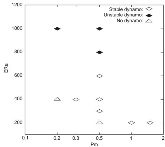
Fig. 1 Diagram of dynamo simulation results. Ordinate represents  $ERa$ , and abscissa  $Pm$ , where  $E$ ,  $Ra$  and  $Pm$  are the Ekman number, the Rayleigh number and the magnetic Prandtl number, respectively. Open diamond represents stable dipolar dynamo, and filled diamond reversing dipolar dynamo, and triangle no dynamo.
