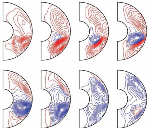
Fig. 2 Time sequence of the dipole field reversal from left to right in top low, then bottom left. Magnetic lines of force are drawn. Parameter values are  $Ek = 10^{-5}$ ,  $Ra = 8 \times 10^7$  and  $Pm = 0.5$ . Red (blue) lines represent counter-clockwise (clockwise) fields.
