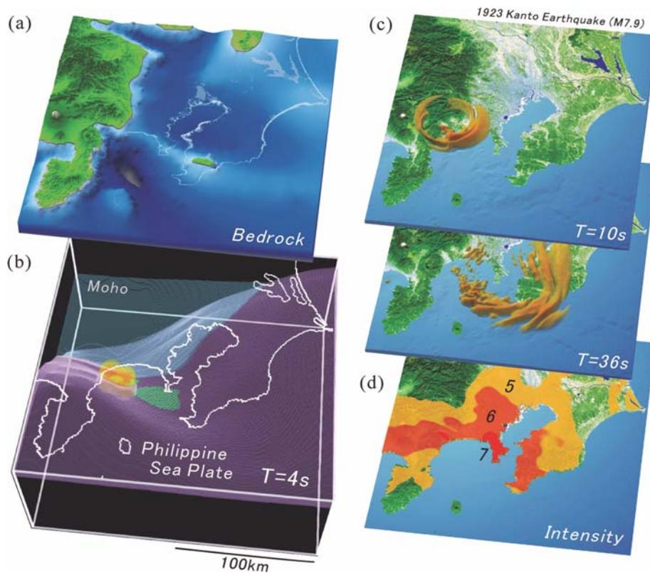
Fig. 3 Structural model of Kanto basin used in the 3D simulation of seismic wave propagation, showing (a) the configuration of sediment/bedrock interface and (b) structure of the Philippine-sea plate. (c) Snapshot of ground motion at 10s, 36s after fault rupture initiation, and (d) intensity distribution derived by the simulation.
