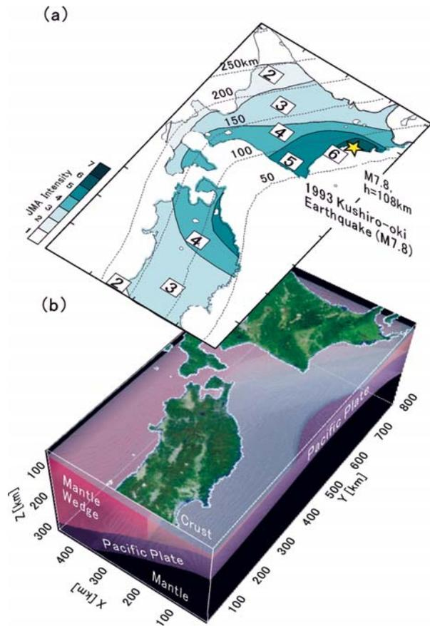
Fig. 1 (a) Intensity distribution of the 1993 Koshiro-oki (M7.8) earthquake, showing anomalous extension of seismic intensity from hypocenter to south for several hundred kilometers along the eastern seaboard. (b) 3D model of the subduction structure beneath northern Japan used in the simulation. The depth of the subducting plate is shown at the top.
