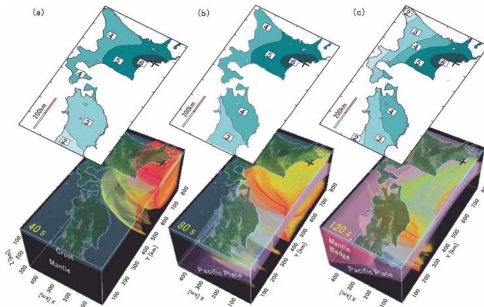
Fig. 2 Snapshot of 3D wavefield from simulation of the 1993 Koshiro-oki earthquake, with (a) laterally homogeneous crust, (b) the inclusion of the high-Q Pacific plate, and (c) the incorporation of a full subduction zone model including the high-Q plate and low-Q mantle wedge. The pattern of intensity from the subduction zone model agrees with observation (Fig. 1).
