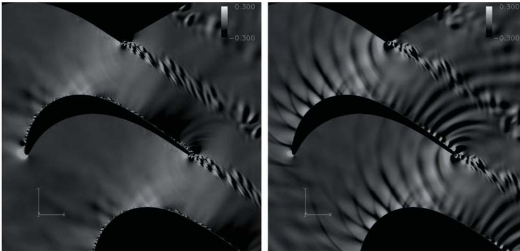
Fig. 3 Instantaneous distributions of static pressure in a turbine-blade cascade with (left) and without (right) incident free-stream turbulence
