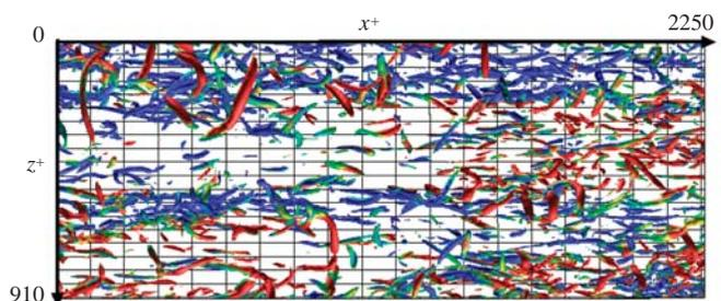
Fig. 4 Plane view of vortices at  $Re_\tau = 1160$ . Iso-surface,  $Q^+ = -0.02$ ; blue to red,  $u^+ = -1$  to  $u^+ = 1$ .
