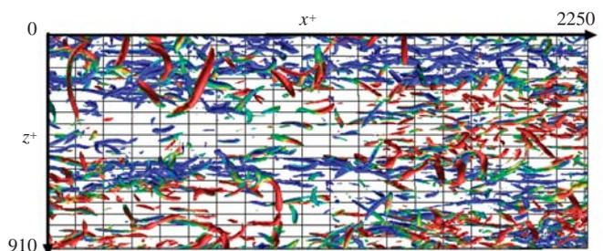
Fig. 4 Plane view of vortices at  $Re_\tau = 1160$ . Iso-surface,  $Q^+ = -0.02$ ; blue to red,  $u^+ = -1$  to  $u^+ = 1$ .
