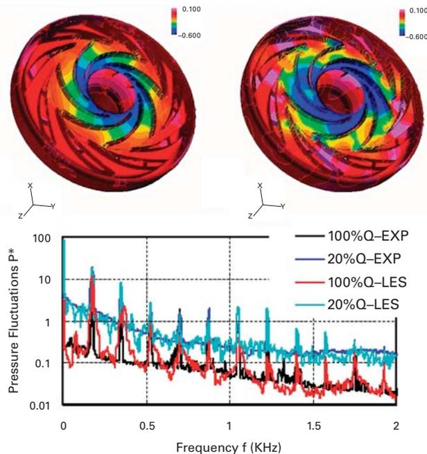
Fig. 2 Instantaneous distributions of static pressure in a centrifugal impeller at two different flow rate ratios (top left: design point, top right: off-design point) and power spectra of the pressure fluctuations (bottom).
