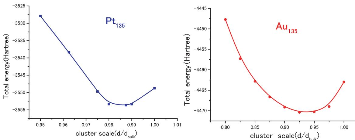
Fig. 3 Optimized cluster sizes of  $Pt_{135}$ , 1.5% contraction, and  $Au_{135}$ , 7% contraction, of fcc nanostructure.
