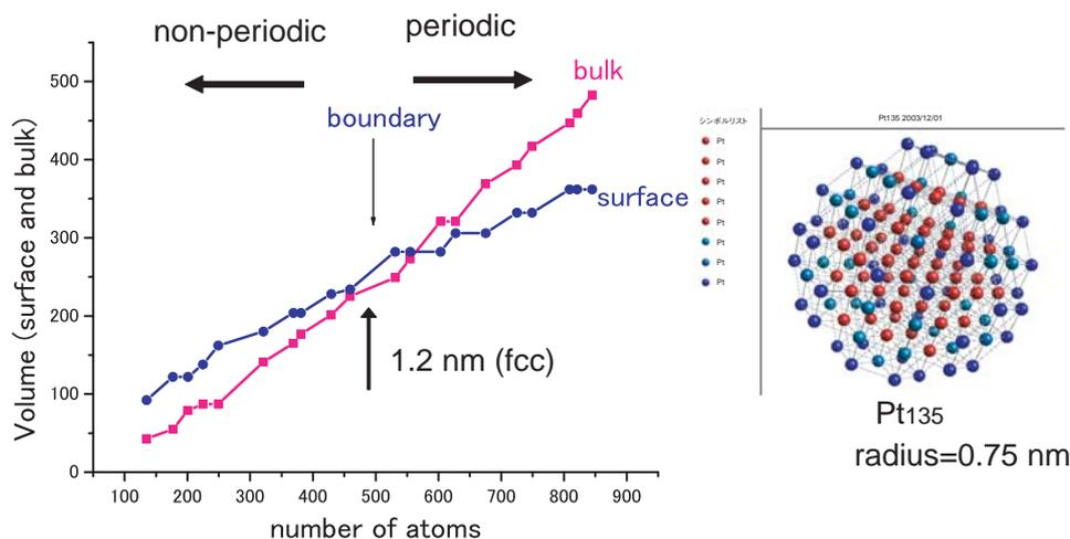
Fig. 2 Critical scale of nanostructure of fcc cluster. 1.2 nm is the radius of the cluster for the boundary.
