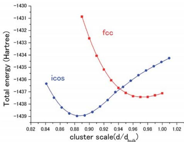
Fig. 5 Energy curves of Pt<sub>55</sub> clusters of fcc and icosahedral symmetry. d<sub>bulk</sub> in the icosahedron is given by the nearest neighbor interatomic distance of twelve vertices.
