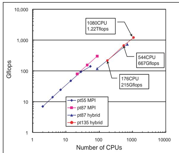
Fig. 1-2 Parallel performance by MPI and hybrid parallelization of LCAO-PS code for various nano-size Pt clusters.
