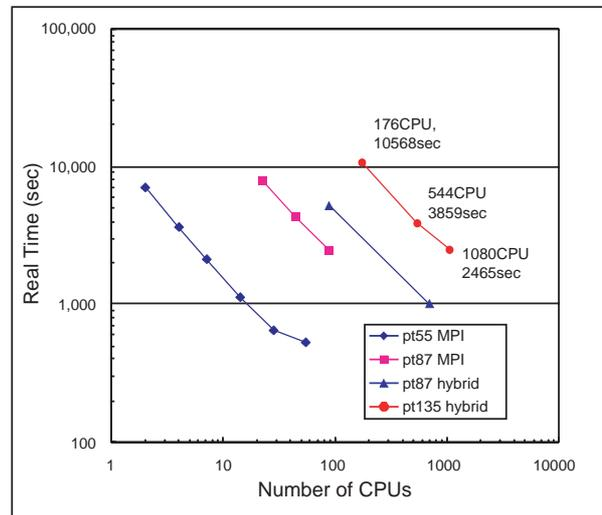
Fig. 1-1 Elapse time by MPI and hybrid parallelization of LCAO-PS code for various nano-size Pt clusters.
