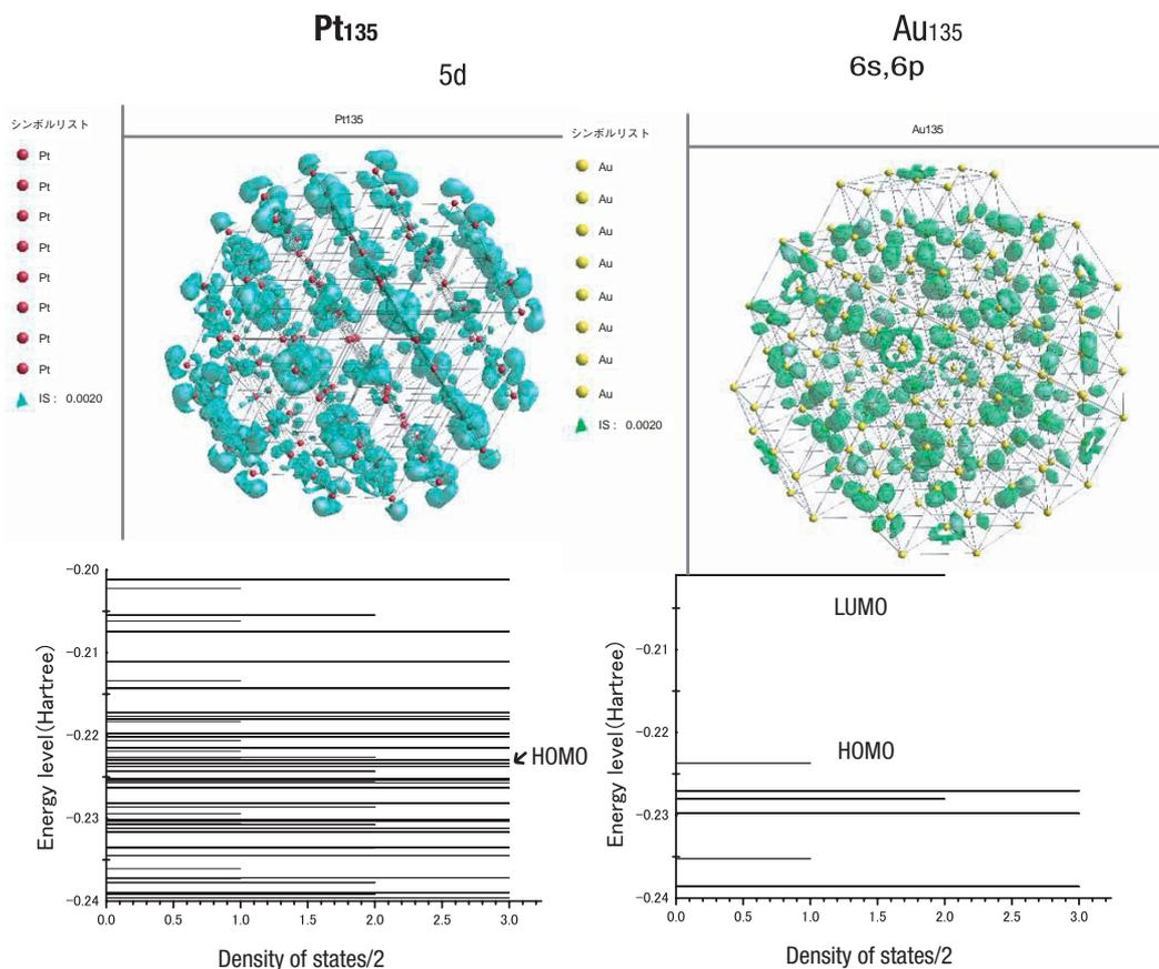
Fig. 4 Energy levels and charge density distribution of highest occupied molecular orbital (HOMO) of Pt<sub>135</sub> and Au<sub>135</sub>. HOMO-LUMO energy gaps are less than 0.01 eV for Pt<sub>135</sub> and 0.6 eV for Au<sub>135</sub>. HOMO states comprise 5d states for Pt<sub>135</sub> and 6s and 6p states for Au<sub>135</sub>.
