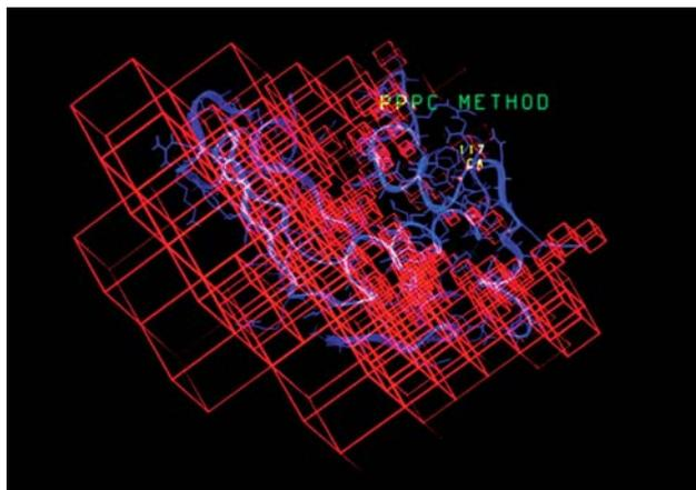
Fig. 1 Particle-Particle and Particle-Cell (PPPC) method. Long-range Coulomb interactions are calculated in the order  $N \log N$  using the PPPC method. This figure shows a space subdivision based on PPPC to calculate Coulomb forces acting to the 117<sup>th</sup>  $\alpha$ -carbon atom of human lysozyme (130 amino acids).
