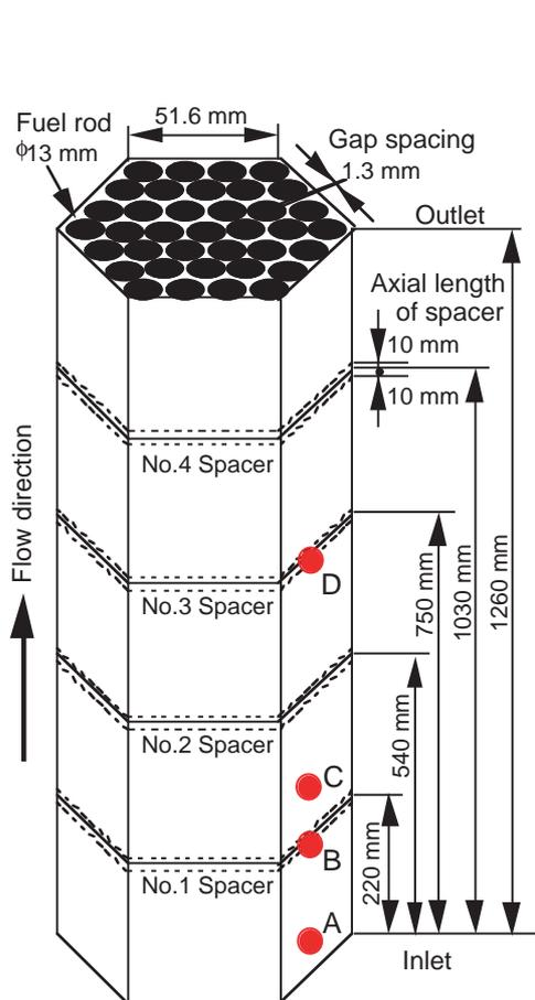
Fig. 1 Outline of three dimensional analytical geometry of a tight-lattice fuel bundle.
