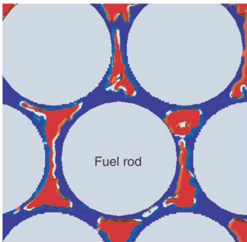
(Blue and red show water and vapor. Void fractions of blue and red are larger and smaller than 0.5, respectively.)
