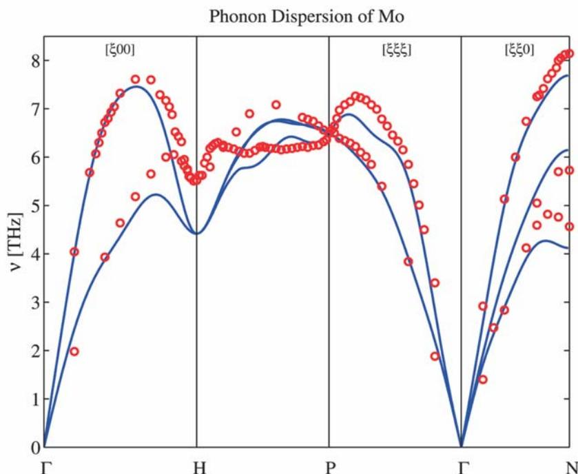
Fig. 2 Phonon dispersion curve of BCC Mo 250 atoms with  $6 \times 6 \times 6$  kpoints.
