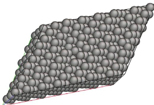
Fig. 1 The BCC Mo supercell consisting of 231 atoms
