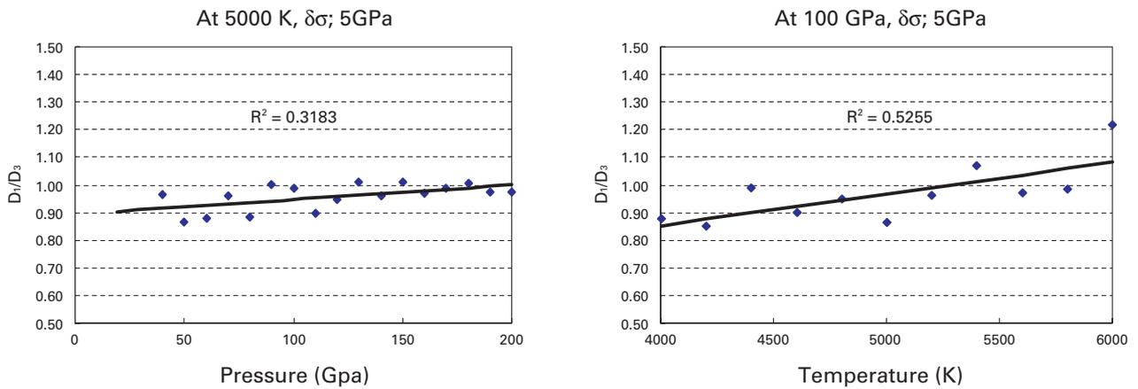
Fig. 2 Simulation results by MD method of anisotropic ratio of diffusion constant  $D_1/D_2$  versus temperature (left) and pressure (right).
