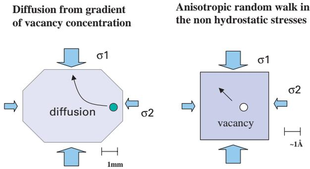
Fig. 1 Comparison of the grain scale deformation with nanoscale rheology controlled by vacancy diffusion. Left; grain scale diffusion creep (NH creep), and right; nanoscale deformation of crystal due to vacancy migration under non hydrostatic stresses.
