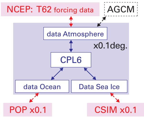
Fig. 7 Schematic diagram of high resolution ocean model (POP) and sea ice model (CSIM) coupling procedure.
