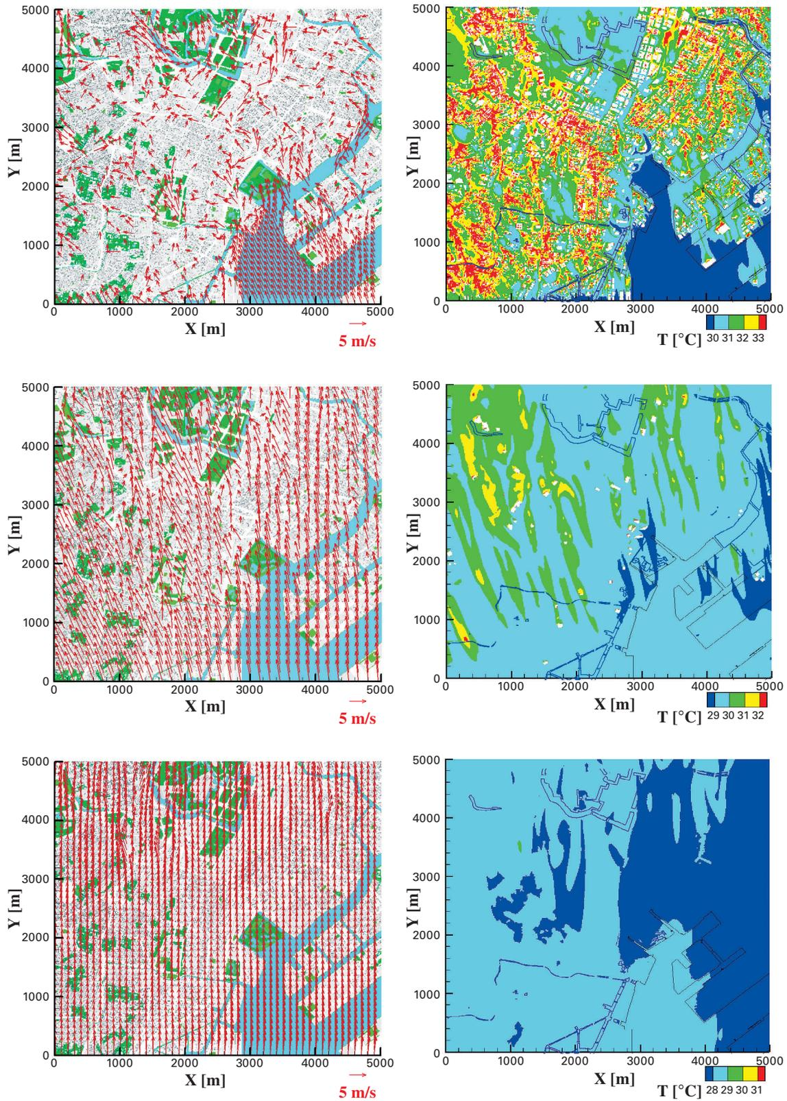
Fig. 3 Distribution of Velocity vectors (left) and air temperature (right).
