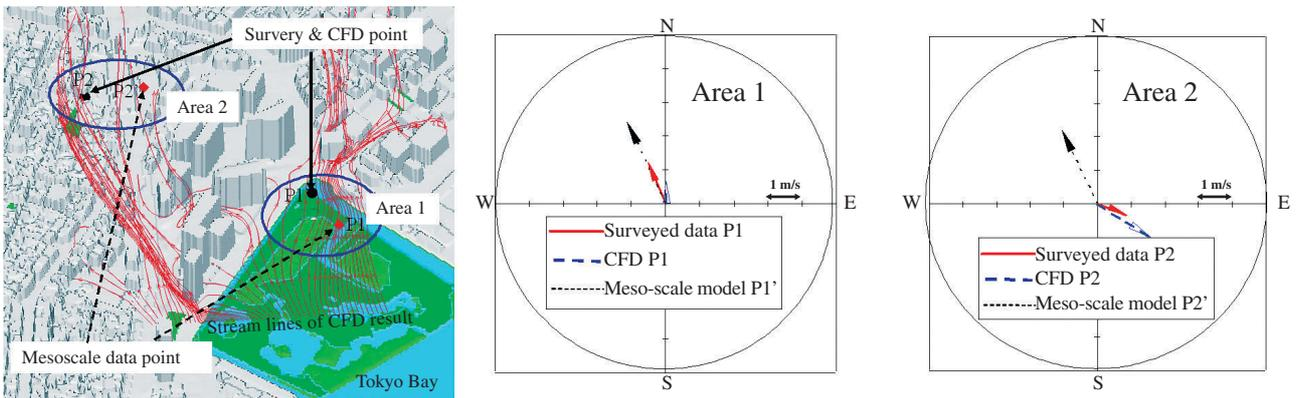
Fig. 4 Wind directions at 14:00: Surveyed result, CFD and mesoscale model.
