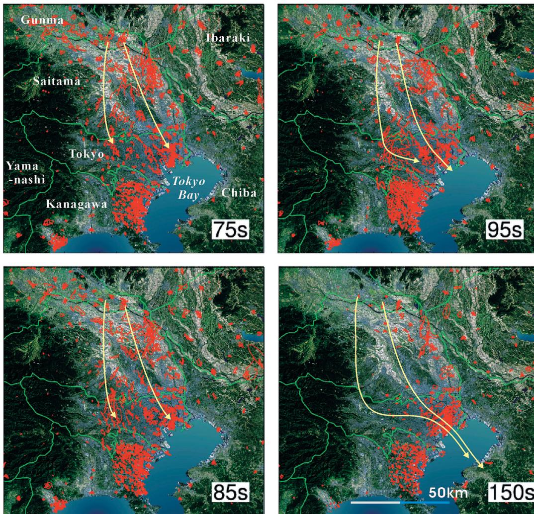
Fig. 2 Particle motion of horizontal ground motions recorded by 459 intensity meters stationed in the Kanto basin and at 268 K-NET and KiK-net stations. The two yellow arrows indicate the estimated major wave propagation paths of the surface waves that affected central Tokyo. The time from earthquake rupture is shown in the bottom right corner.
