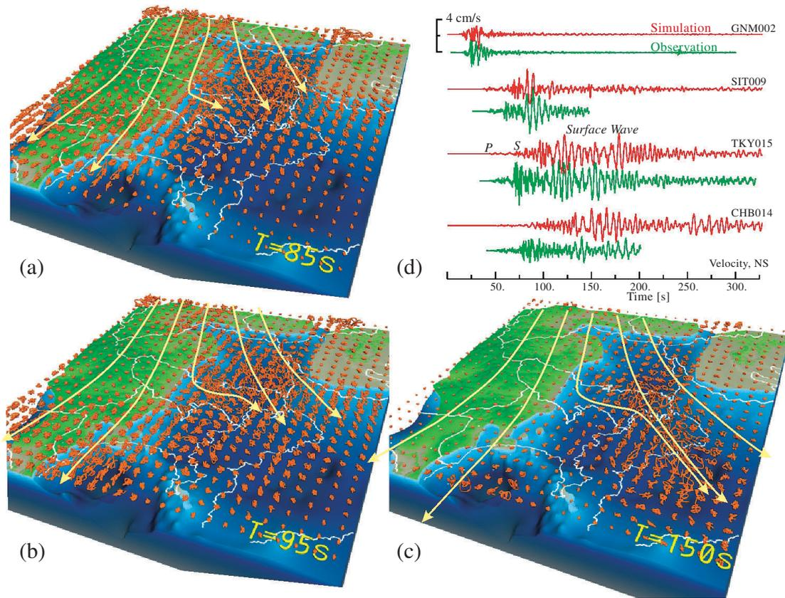
Fig. 3 (a-c) 3D view of simulated particle motions and ray path of derived surface waves. Time from origin is shown in the bottom right corner of each figure. (d) Comparison of simulation waveforms (orange) and observed waveforms (green) of ground velocity motions.
