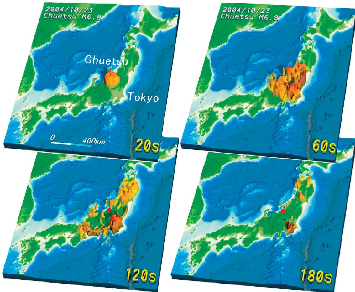
Fig. 1 Distribution of ground motion following the Niigata-ken Chuetsu earthquake, Japan. The amplitude of ground velocity motions derived by interpolation of dense seismic array recording is displayed in each sequence of snapshot at  $T = 20, 60, 120,$  and  $180$  s after rupture.
