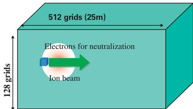
Fig. 2 Three-dimensional simulation model for ion beam injection.
