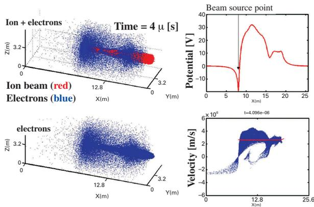
Fig. 3 Spatial distribution of beam ions and electrons for charge neutralization in left panels. Potential and plasma velocity versus the  $x$  axis in right panels for the case of  $v_{\text{the}}/v_{\text{ion\_beam}} = 0.07$ .
