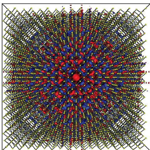
Fig. 4 The wave function of As-donor state in silicon. An As atom is substituted for the center Si atom, and the super-cell contains 5,832 atoms. The blue and red regions show the sign of the wave function.
