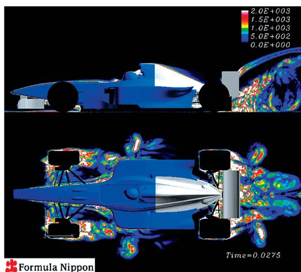
Fig. 3 Instantaneous vorticity distribution around a formula car obtained with the large-scale LES.
