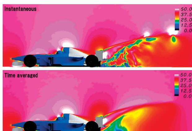
Fig. 2 Instantaneous and time averaged velocity distribution around a formula car obtained with the large-scale LES.
