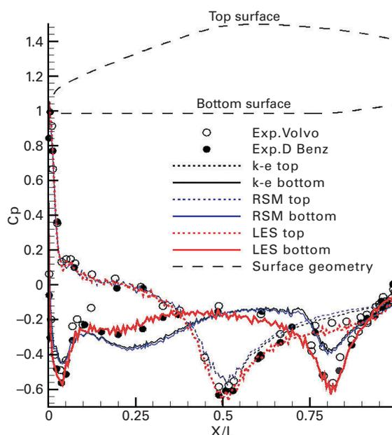
Fig. 1 Surface pressure distribution of ASMO model (Comparison with LES, RANS, and experimental data).
