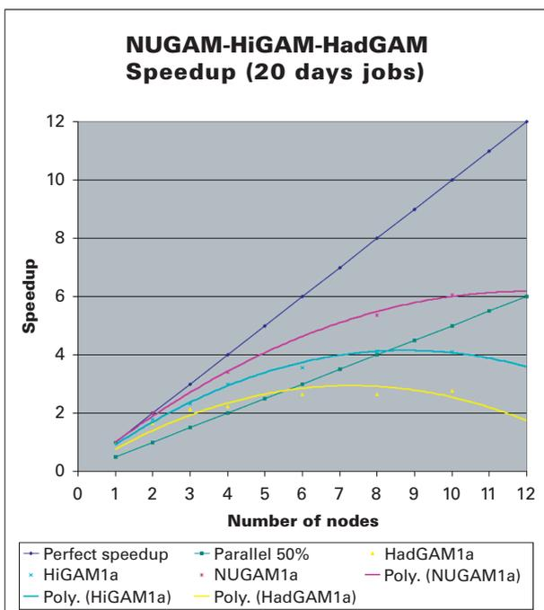
Fig. 1 The speedup factor of individual members of the UJCC model chain on the Earth Simulator: HadGAM (N96), HiGAM (N144) and NUGAM (N216), as dependent on the number of nodes used in the integration.
