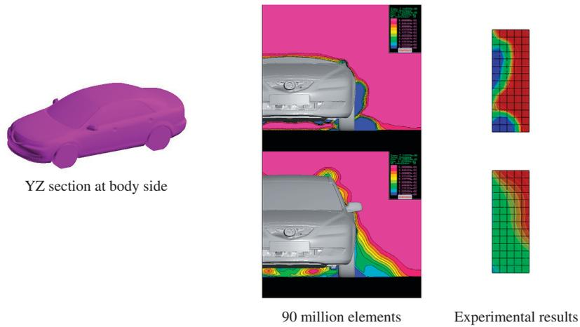
Fig. 5 Pressure distribution: YZ section at body side.
