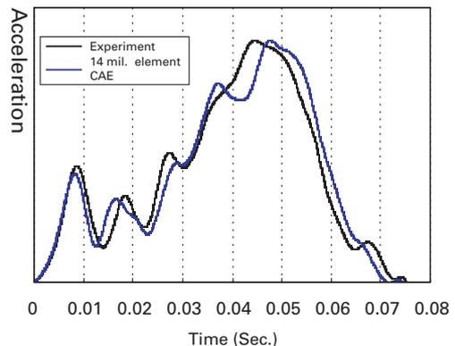
Fig. 2 Acceleration-Time Graph (Front Passenger Seat).
