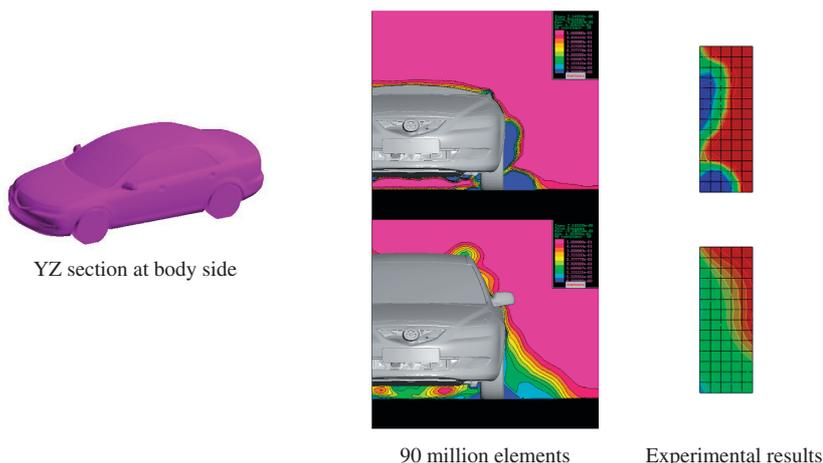
Fig. 5 Pressure distribution: YZ section at body side.
