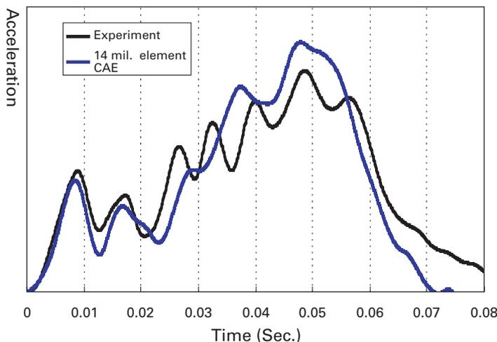
Fig. 1 Acceleration-Time Graph (Driver's Seat).
