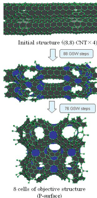
Fig. 5 Snapshot of isomerization (Structure consisting of 144 atoms per cell).
