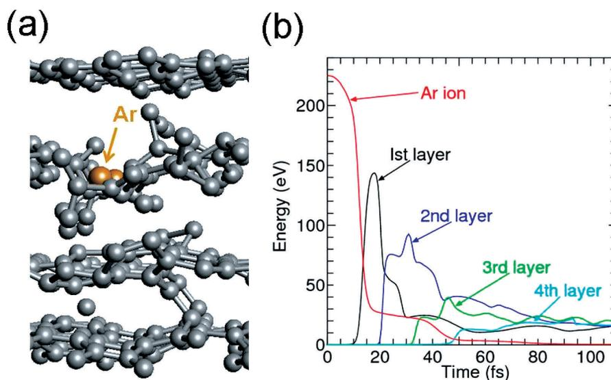
Fig. 2 (a) The modified structure of graphene sheets irradiated by an  $\text{Ar}^{8+}$  ion with incident energy of 225 eV. (b) The corresponding distribution of kinetic energies of Ar ions, of C atoms in the 1<sup>st</sup>, 2<sup>nd</sup>, 3<sup>rd</sup>, and 4<sup>th</sup> layers, as a function of time.
