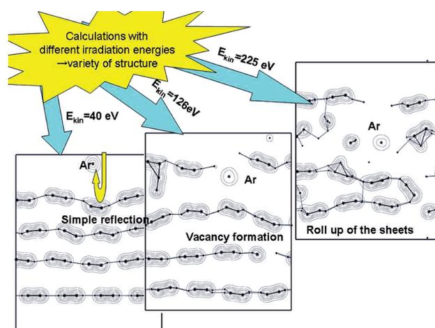
Fig. 1 Varieties of structures obtained upon  $\text{Ar}^{8+}$  irradiation with several incident energies denoted in each panel. The charge contour maps are also shown indicating semi-neutralization of  $\text{Ar}^{8+}$  ion in each case.
