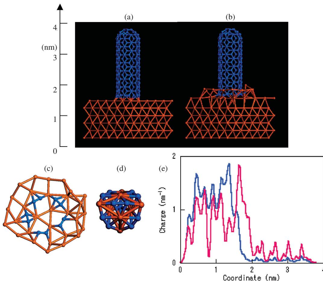
Fig. 3 (a) Simple and (b) stabilized atomic structures of the contact between carbon nanotube (CNT) and titanium (Ti). The blue and orange spheres represent C and Ti atoms, respectively. (c) Nanoparticle-like structure at the root of the CNT and (d) the  $\text{Ti}_8\text{C}_{12}$  nanoparticle. (e) Initial (blue) and stabilized (red) charge distributions near the Fermi level along the tube direction.
