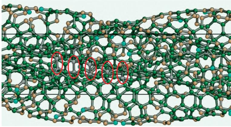
Fig. 7 The  $sp^3$  hybridization between CNTs.
