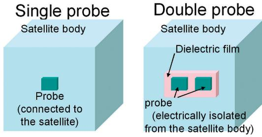
Fig. 2 Single- and double- Langmuir probe.
