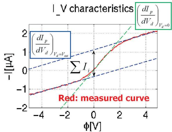
Fig. 6 Current-Voltage curve obtained for the double probe.
