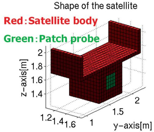
Fig. 3 Simple Reimei model for simulation.
