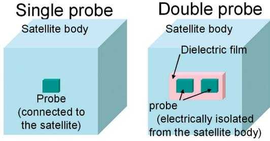
Fig. 2 Single- and double- Langmuir probe.
