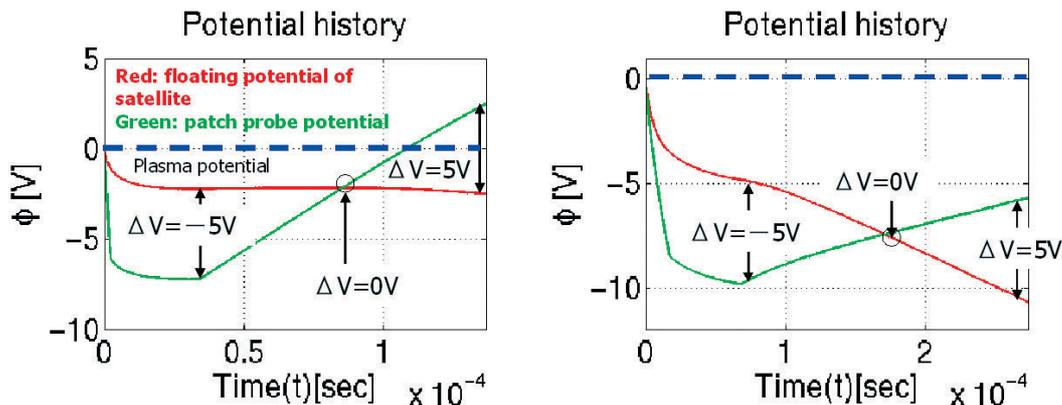
Fig. 4 Potential variation of single patch probe in the plasma environment without electron flux (left), and with electron flux (right).
