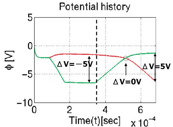
Fig. 5 Potential variation of double probe.
