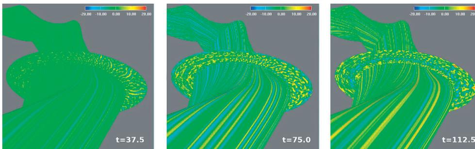
Fig. 2 Snapshots of the electrostatic potential perturbations at  $t=37.5 L_n/v_t$  (left),  $75.0 L_n/v_t$  (middle), and  $112.5 L_n/v_t$  (right) obtained by the GKV simulation of ITG turbulence in a helical system with  $L=2$  and  $M=10$  like the LHD. The equilibrium magnetic field is given by a single-helicity model configuration.
