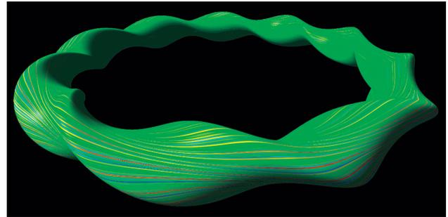
Fig. 1 A whole picture of a helical system of  $L=2$  and  $M=10$ , where the innermost toroidal magnetic surface is plotted. Here,  $L$  and  $M$  denote the poloidal and toroidal periodicities of the major helical component of the confinement field. Red and blue colors represent positive and negative electrostatic potential perturbations of the ion temperature gradient mode resulted from the GKV simulation.
