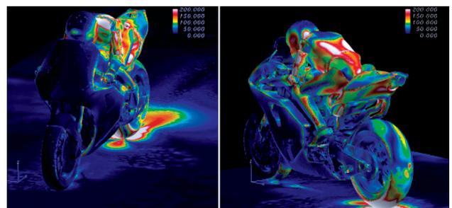
Fig. 2 Snapshots of the pressure fluctuation on the surface of the racing motorcycle (SUZUKI GSV-R) and rider.
