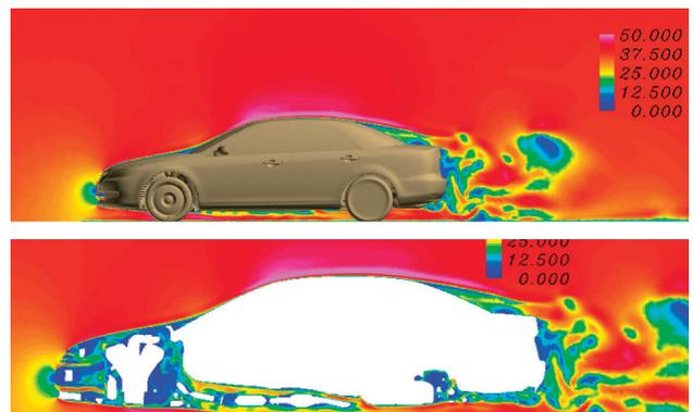
Fig. 3 Snapshots of the velocity distribution around the commercial sedan (MAZDA Atenza).
