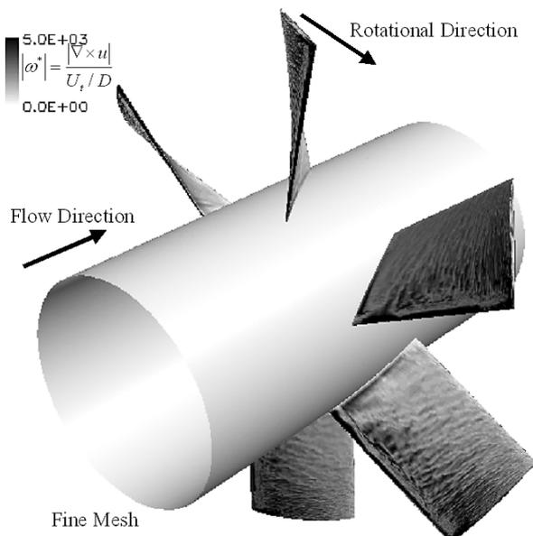
Fig. 4 Distribution of vorticity magnitude on hub and rotor blade surfaces.
