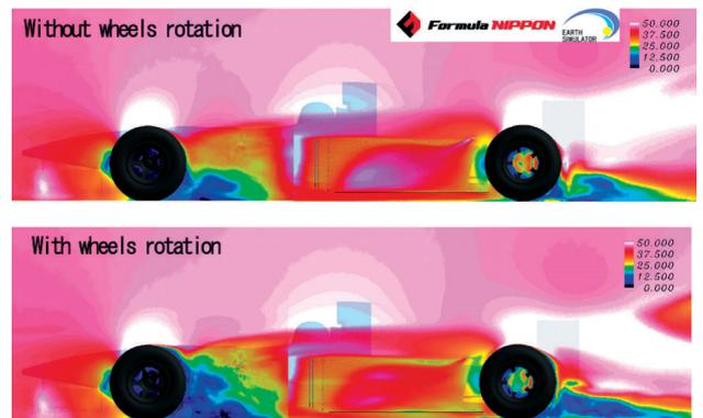
Fig. 1 Snapshots of the velocity distribution around a formula car with (below) or without (above) wheels rotation.
