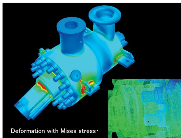
Fig. 7 Self-gravity analysis of 100 million D.O.F high-pressure pump model.
