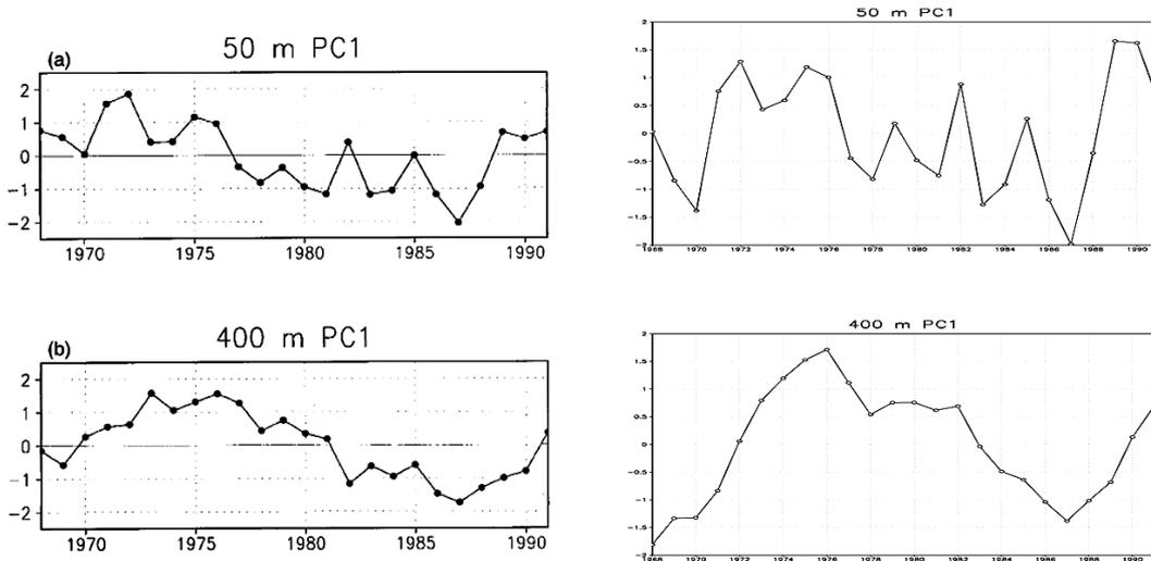
Fig. 2 (Left top) the first EOF component of annual mean sea temperature at 50 m over the region (150E–120W, 24N–56N) due to observation (Deser et al., 1999) and (right top) model results. (Left bottom) The first EOF component of the annual mean sea temperature at 400 m depth due to observation and (right bottom) model results. Amplitudes are normalized due to standard deviations.
