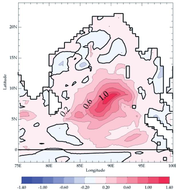
Fig. 2 15 days mean SST difference: 301 levels minus 31 levels in April 1992, Units=°C.
