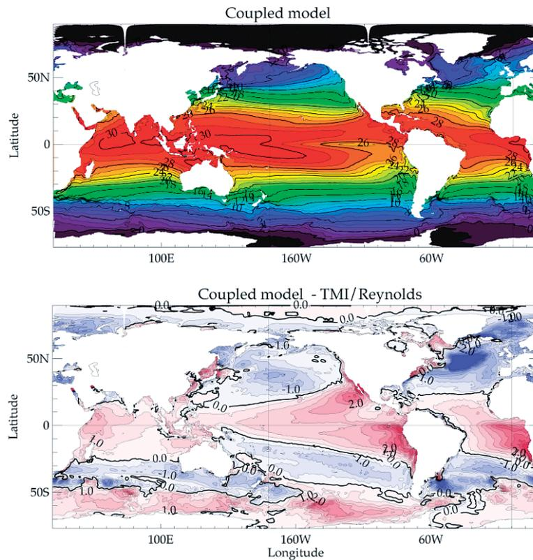
Fig. 3 Upper: model SST 50-year climatology. Lower: differences with observations (TMI and Reynolds). Units= $^{\circ}\text{C}$ .
