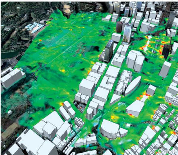
(b) Temperature distribution is shown at the height of 7.5m from the ground.
