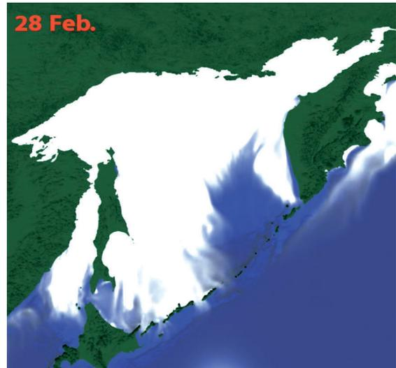
Fig. 7 Snapshot of concentration distribution on 28<sup>th</sup> February using MSSG coupled to the introduced sea ice model.
