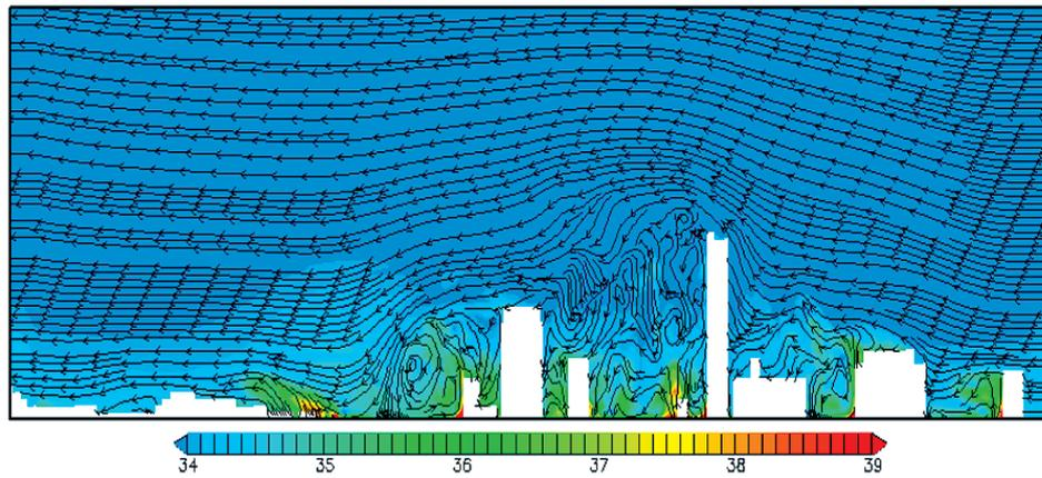
Fig. 3 Wind stream function and temperature distribution in for the vertical.
