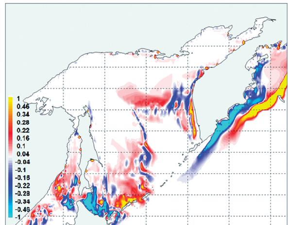
Fig. 8 Comparison of distribution sea ice concentration between simulation result using sea ice collision effects and results without collision effects.
