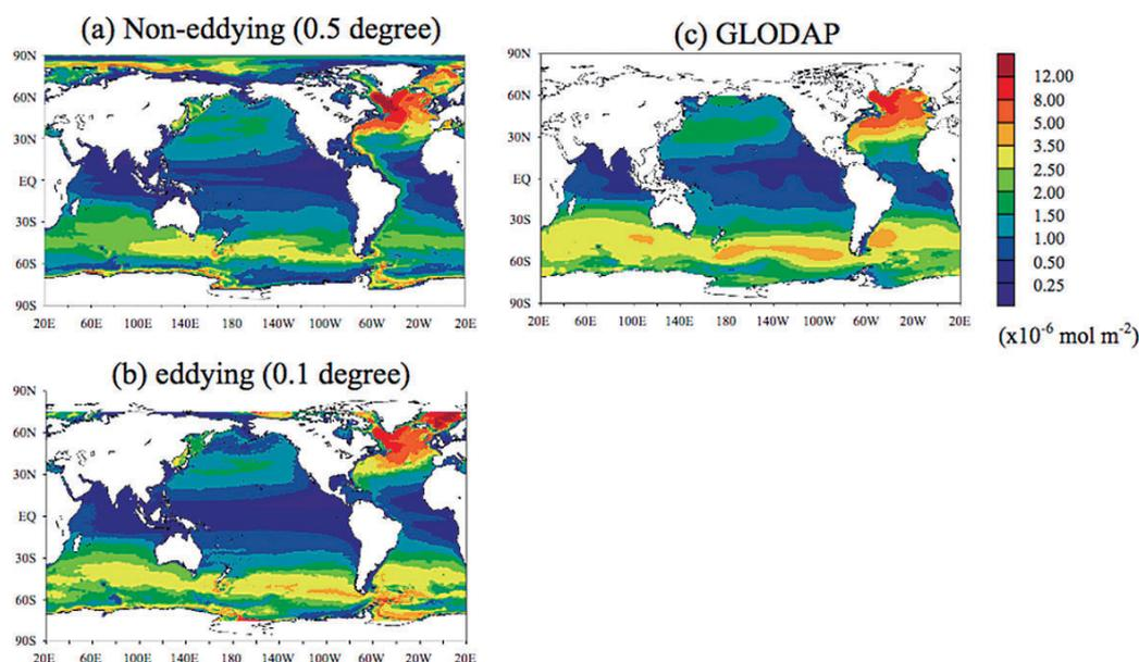
Fig. 2 Horizontal distribution of CFC-11 inventory from the model with 0.5 degrees resolution (a), 0.1 degrees (b), and the data-based estimation (c).
