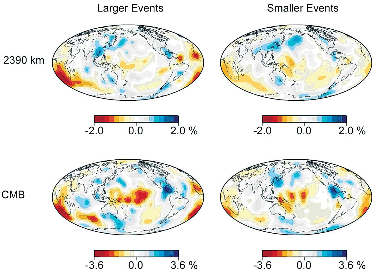
Fig. 2 The SH velocity models at 2390 km (top) and CMB (bottom) obtained in the previous study (left; SH18CE) and this study (right).
