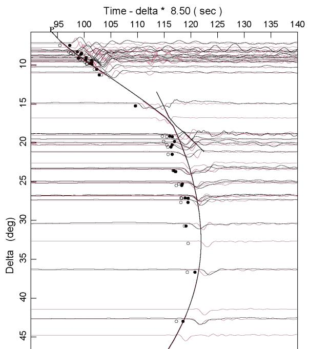
Fig. 4 Comparison of synthetic seismograms (red) and observed seismograms (black). Vertical component displacement seismograms for P-arrivals are shown. Observed traces are low-pass filtered at 4 sec. Solid curve in the figure shows theoretical travel time of Iasp91 model. Solid circles are observed arrival times of P-wave and open circles are theoretical ravel times by GAP-P1.
