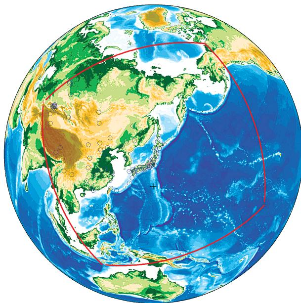
Fig. 3 Black plus sign represents epicenter of June 3, 2002 Bonin earthquake. Blue circles show locations of stations. Red curves show boundary of the one chunk at the surface of the Earth used in the computation.
