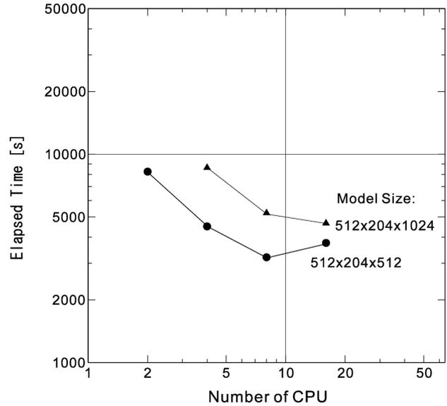
Fig. 1 Parallel performance of the parallel 3D Navier-Stokes simulation in terms of the elapsed time of the tsunami simulation as a function of CPU numbers, and for different scales of the simulation model.
