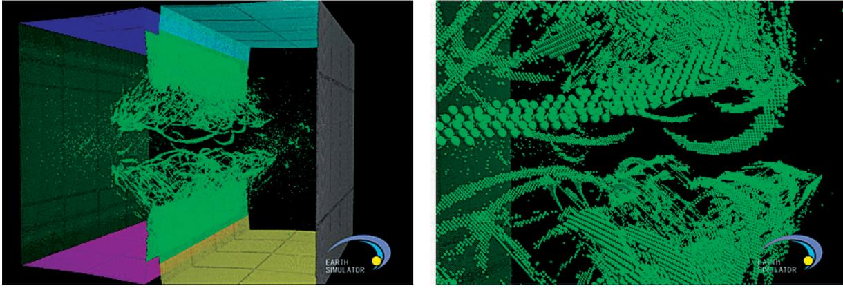
Fig. 7 Molecular dynamics simulation of fracture in Lennard-Jones material. Only atoms of larger potential energy are drawn to show dislocations developing from the tips of cracks. Right panel is a zoom-in view of left.
