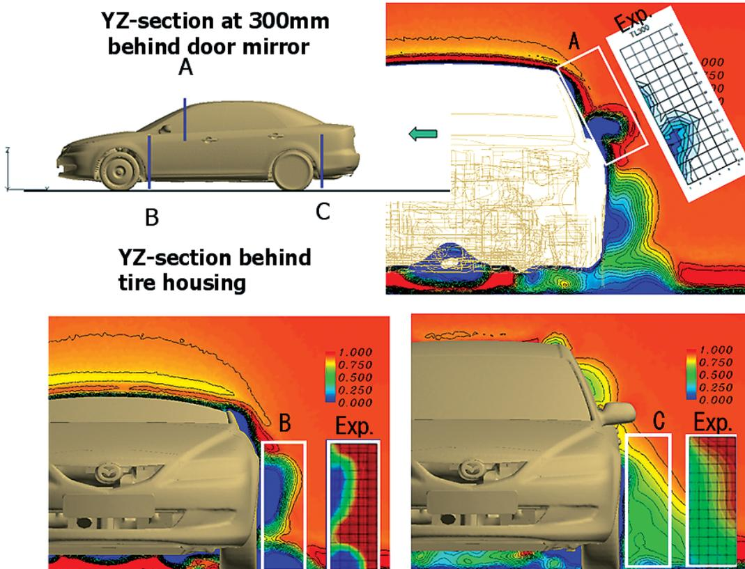
Fig. 1 Flow structures on the side of a vehicle (total pressure distributions) and its comparison with the wind-tunnel experiments.
