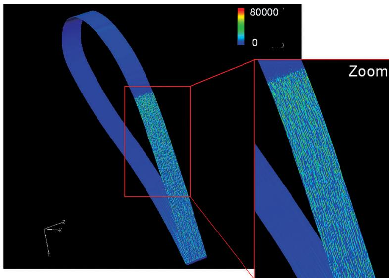
Fig. 6 Magnitude of vorticity distribution on the blade's surface.
