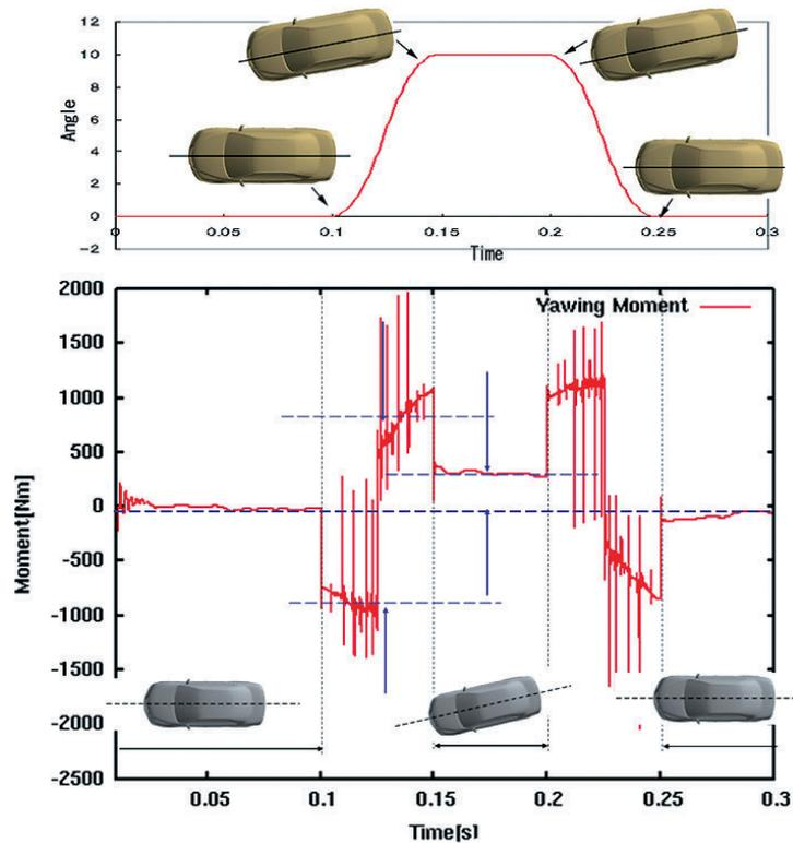
Fig. 2 Time history of the vehicle yawing angle (above) and the yawing moment obtained (below).
