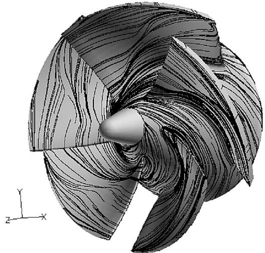
Fig. 5 Stream lines on rotor blades (designed point).
