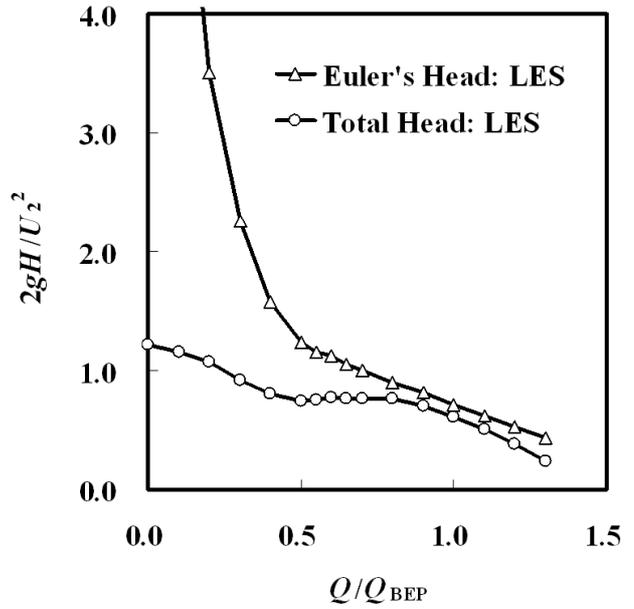
Fig. 4 The Euler head and total head computed by LES.
