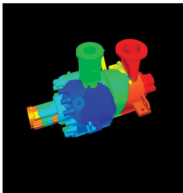
Fig. 9 Domain decomposition of the model (32 domains).
