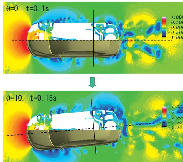
Fig. 3 Snapshots of the pressure distributions around the vehicle during the dynamic yawing-angle change.
