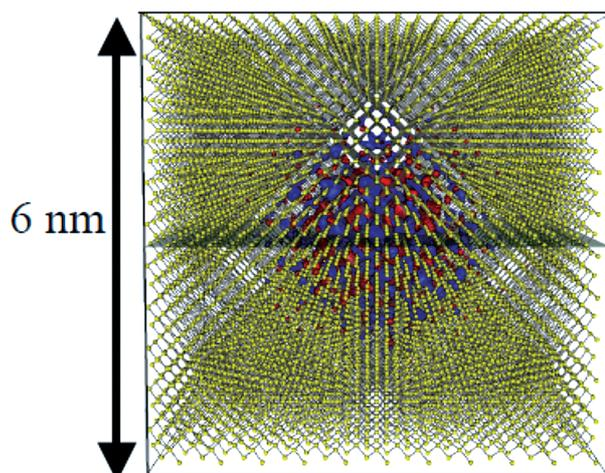
Fig. 11 The wavefunction of the As-donor state in silicon. The yellow balls indicate 10,648 Si atoms in the super-cell, and an As atom is substituted for the center Si atom. The blue and red regions indicate the sign of the donor wavefunction.
