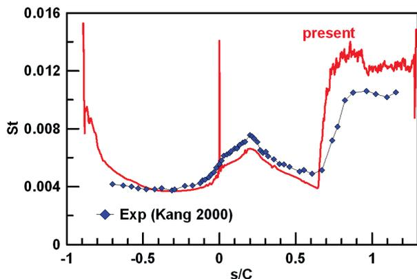
Fig. 7 Stanton number distribution on the blade's surface.
