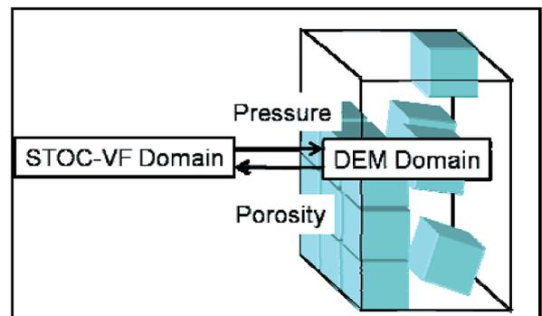
Fig. 4 Relation between DEM and STOC-VF.
