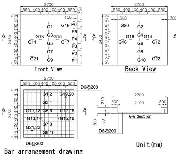
Fig. 7 Plan of reinforced concrete wall.
