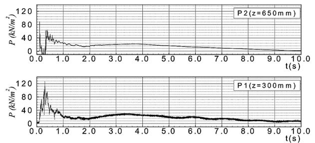
Fig. 8 Time history of tsunami pressure on the wall.
