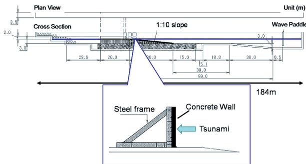
Fig. 6 experimental set up.
