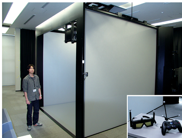
Fig. 4 A CAVE system "BRAVE" installed in ESC.
