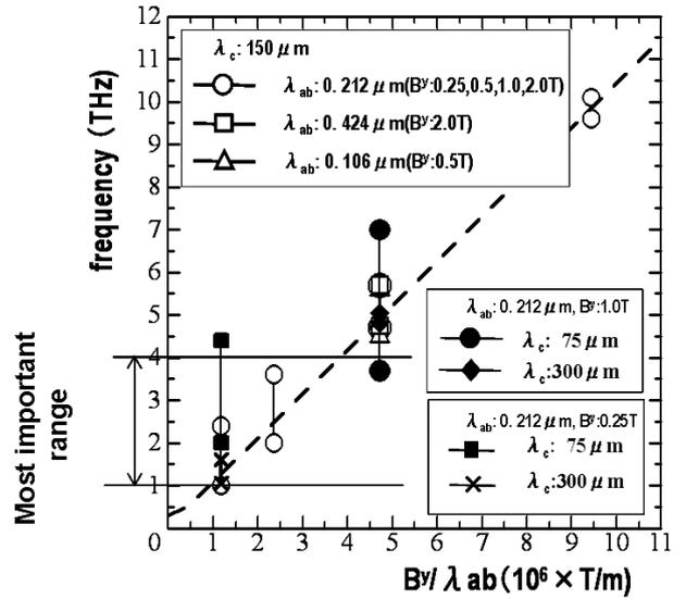
Fig. 2 Relation between frequency of excited Josephson plasma and parameter  $B^y/\lambda_{\text{ab}}$  with changing  $\lambda_c$ . Symbols connected by line shows the range of frequency of excited Jpsephson plasma. Dash line shows an analytical solution of linearized gauge-invariant phase difference equation.
