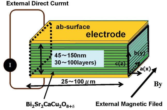
Fig. 1 Schematic diagram of the device generating terahertz waves.  $\text{Bi}_2\text{Sr}_2\text{CaCu}_2\text{O}_{8+\delta}$  forms IJJ. The device is consists of HTC crystal and electrodes. The green part shows the IJJ sandwiched by electrodes. An external current flows uniformly in the junctions in the direction of the  $z$  axis. An external magnetic field is applied to  $y$ -direction.
