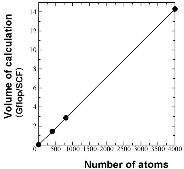
Fig. 3 Relation between number of atoms and volume of calculation for DFTB model.
