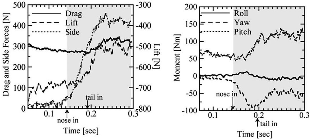
Fig. 1 Time history record of aerodynamic forces on the vehicle subjected to sudden crosswind (left: forces, right: moments). Shaded area indicates when the vehicle is in the crosswind region.
