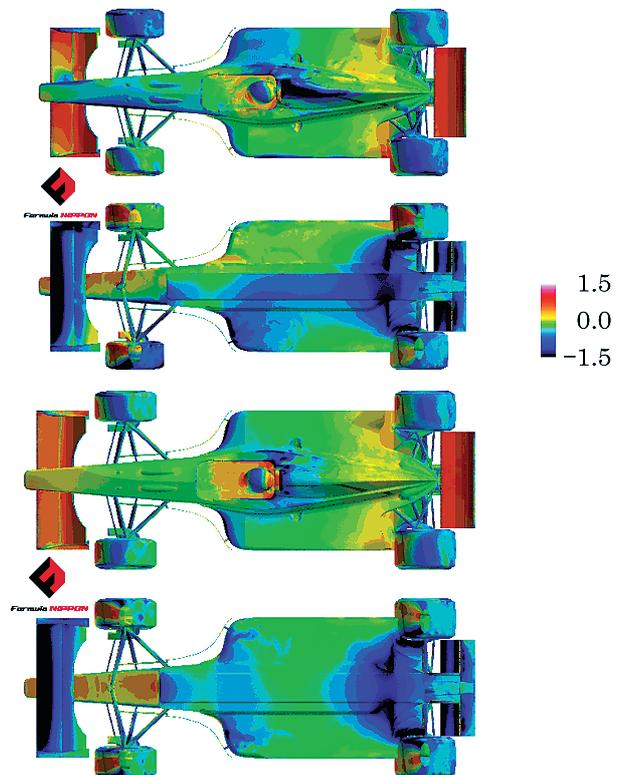
Fig. 3 Snapshots of surface pressure coefficient  $C_p$  on car body at  $T = 0.14$  (above) and  $0.20$  (below) sec.
