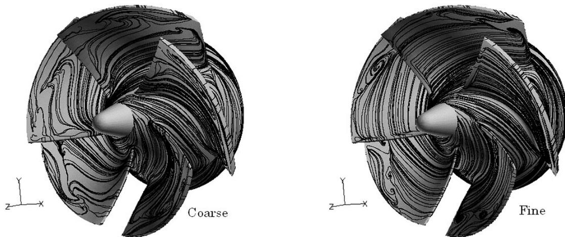
Fig. 4 Surface-limited streamlines of time-averaged flow on impeller blade surfaces at 55% flow rate [6].
