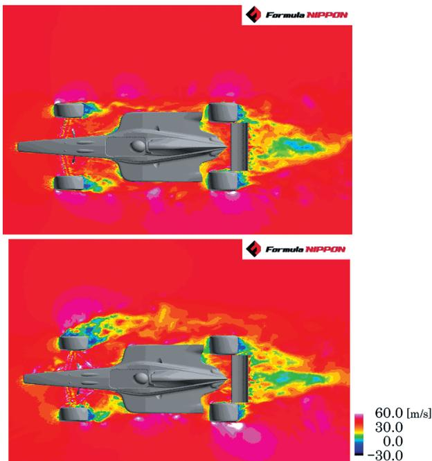
Fig. 2 Snapshots of streamwise velocity at  $T = 0.14$  (above) and  $0.20$  (below) sec.
