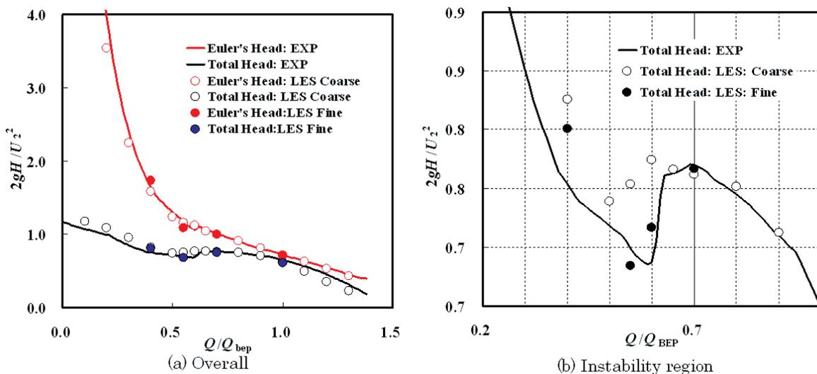
Fig. 5 Performance curve of pump predicted by LES [6].
