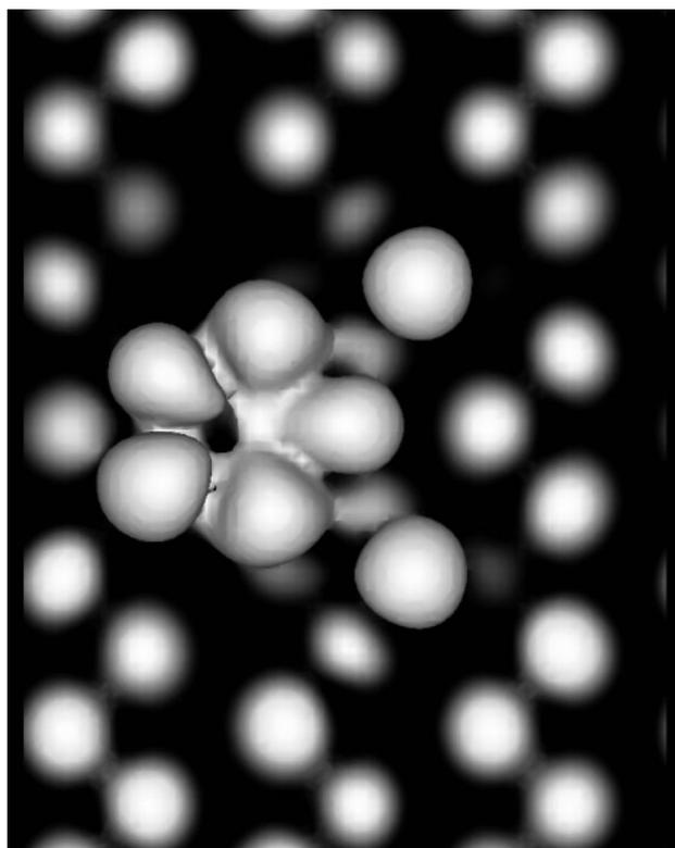
Fig. 7 Scanning tunneling microscope image of proposed model of five-member ring structure on Si(110) surface [7].
