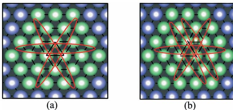
Fig. 2 The relaxed core structure of a screw dislocation without (a) and with one hydrogen atom (b).
