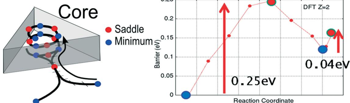
Fig. 6 A diffusion path and its energy landscape from the trapping lattice site to the core of a screw dislocation.
