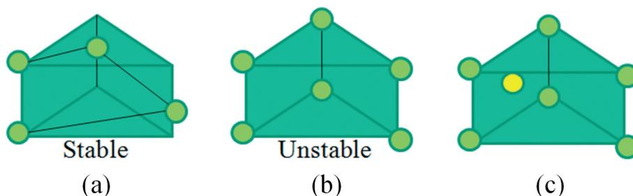
Fig. 3 Atomic configurations of one unit layer for the core region of a screw dislocation.
