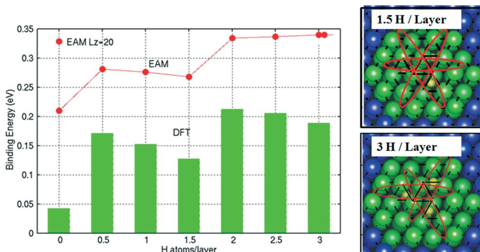
Fig. 5 The binding energy of hydrogen as a function of the number of hydrogen atoms per unit layer.
